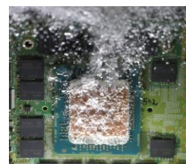
Boiling NOVEC at an Intel Xeon Phi
