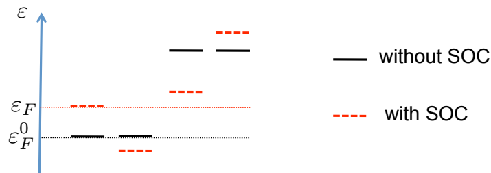
Figure 2.14: Change in the Fermi energy after adding 1st-order SOC contribution. \varepsilon_F is the Fermi energy with SOC, whereas \varepsilon_F^0 is the Fermi energy without SOC.
