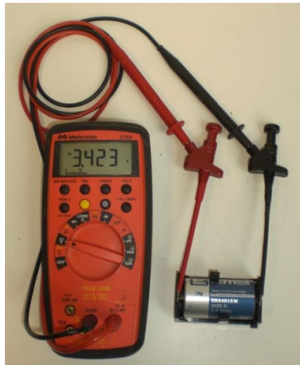
Figure 12: Measuring battery voltage with activating tool
