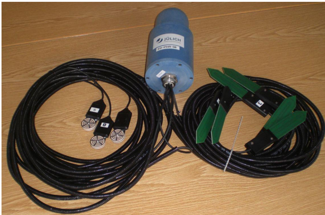
Figure 1: End Device with 6 smt100 sensors and 3 Teros 21 sensors
