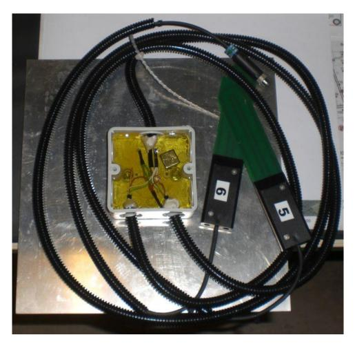
Because the SMT sensors have the SDI-12 bus, they can be wired together in parallel, so only one cable has to be connected with the End-Device above the surface and has to be buried under the baseplate to be protected from the farmers tools.
