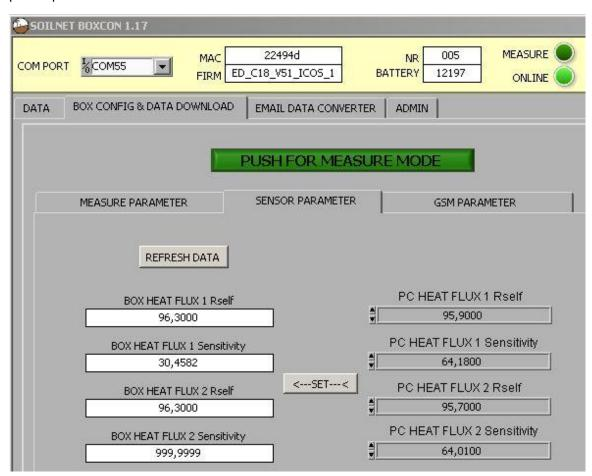
After setting the data press the button "**Push for Measure Mode**" to return to normal operation.
