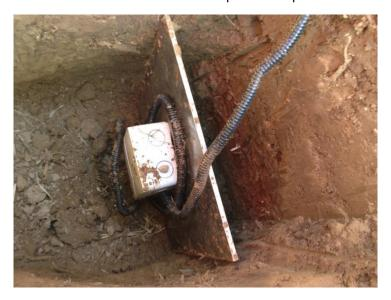
Soil moisture sensors number 1 to 4 are inserted
