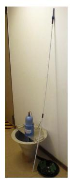
Here you see the rod antenna connected to a standard End-Device.
