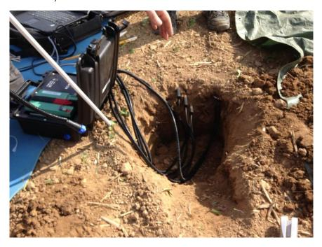
The case is left on the ground while measuring period. The four sensors near the surface as well as the heat flux plate have to be removed while field working.
