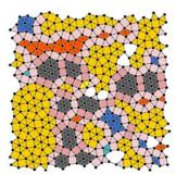
Two-dimensional quasicrystal structure consisting of fullerenes with twelvefold symmetry
