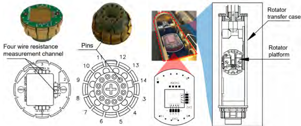
(a) Standard puck for resistivity measurements. (b) Horizontal rotator probe for resistivity measurements.
