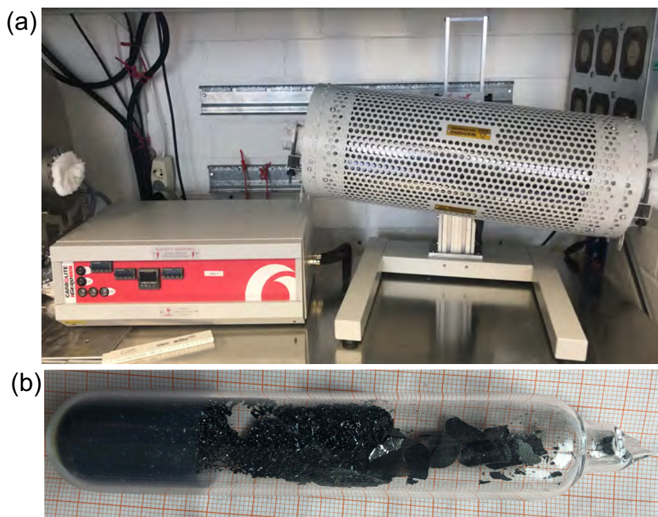
Figure 3.4: Equipments of the crystal growth from CVT method in this PhD work. (a) Three zone tube furnace for the crystal growth from CVT in this PhD work (Carbolite Gero). (b) A silica ampoule with \alpha - \text{RuCl}_3 single crystals after growth inside.
