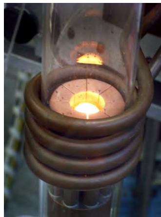
Figure 3.2: Photo of the melting process of the material in the cold crucible induction melting [taken from [95]].
