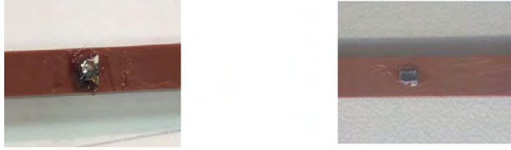
Figure A.6: Photos of the \text{MnFe}_4\text{Si}_3 samples that were used in the magnetization measurements parallel to a -axis (left) and parallel to c -axis (right).
