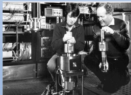
Above: Exchange of Fermi rotors at ISIS (UK): 7 kg; 36,000 rpm
