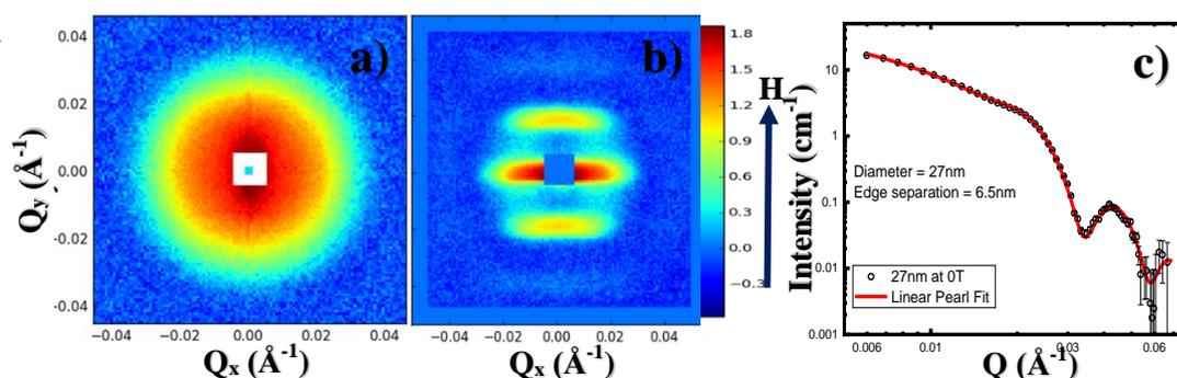
Figure 1: SANS pattern at room temperature in H=2.2T (similar concentration) of a) 20nm b) 27nm NP (colour bar in logscale) c) Radially averaged SANS of 27nm NP's in 0T at room temperature (red line linear pearl model fit)
