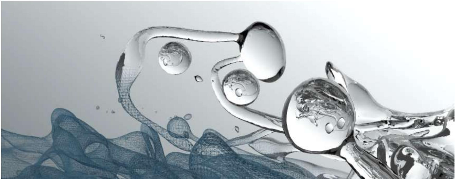
rendered with Blender from a DNS of a diesel injection spray of ITV, RWTH Aachen University
