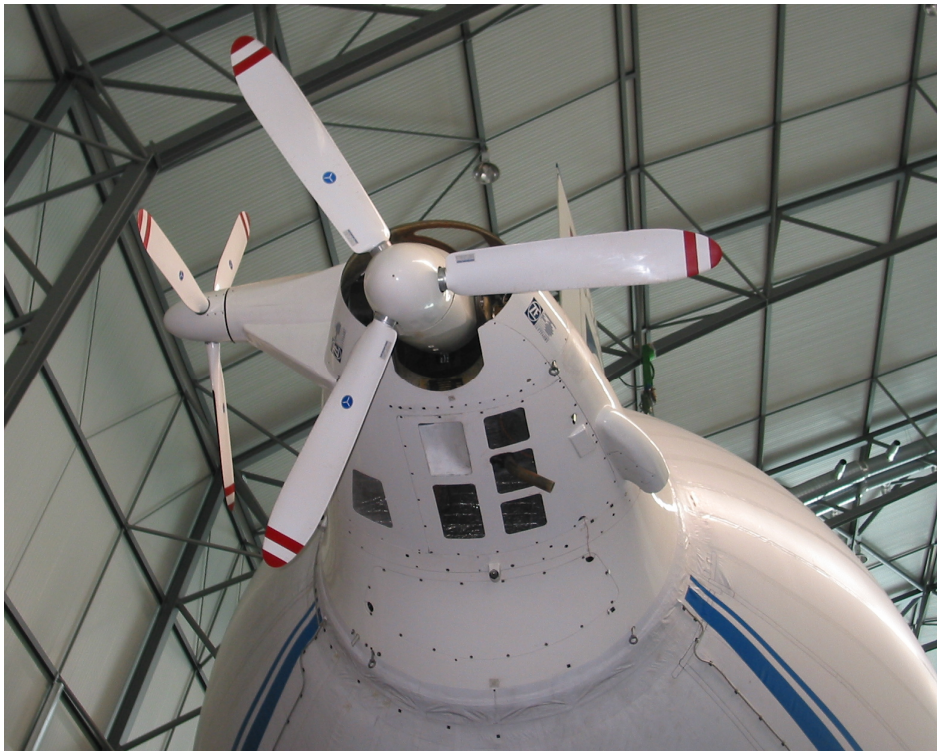
Figure 5: Rear swivelling propulsion engines including electrical power generation units.
