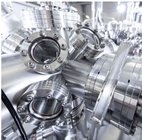
A NanoCluster, housed in the HNF, in which core components of the hybrid qubit are manufactured.
